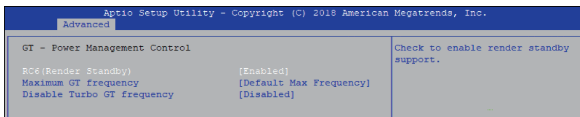
Figure 4 3-2-2 : GT – Power Management Control
